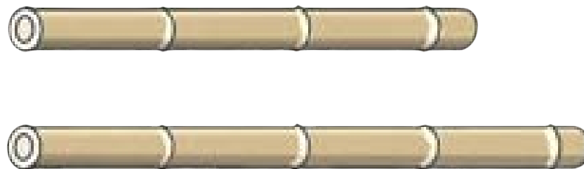
Figure 28. The poles are sectioned to the required lengths for treatment
