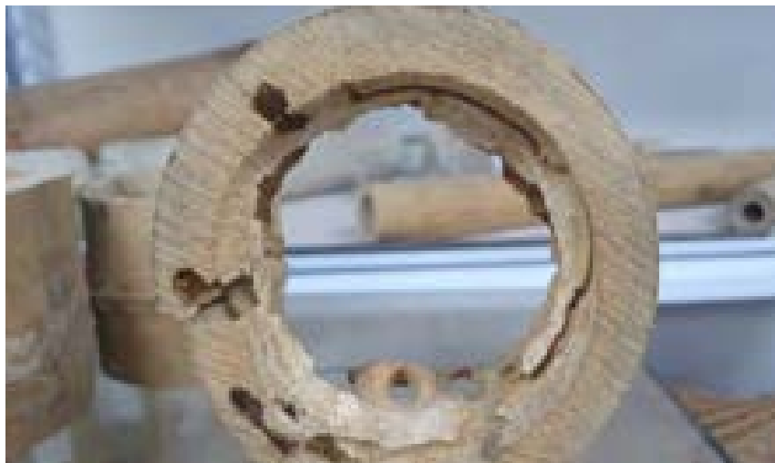
This cross-section of the bamboo culm shows the damage inside caused by the longhorn beetle.
