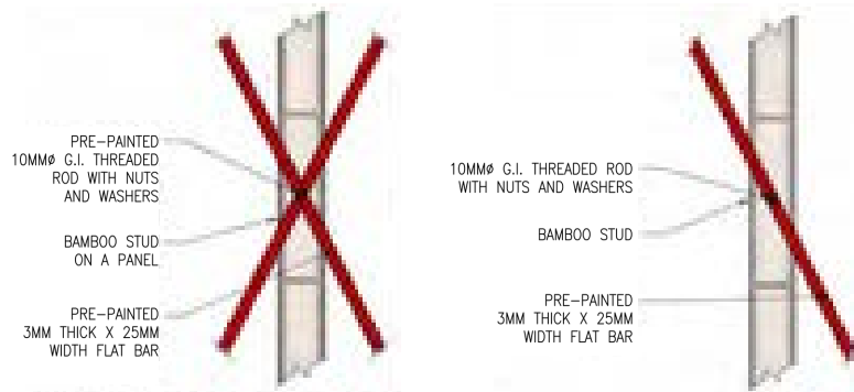
TWO FLATBAR CONNECTION DETAIL
