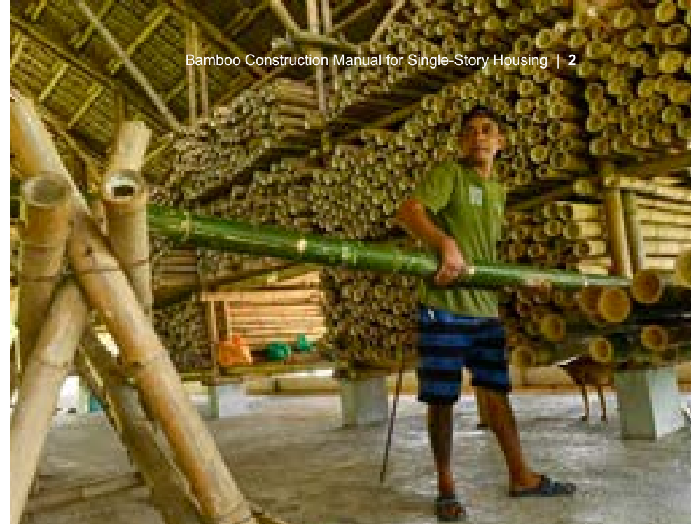
Node punching, part of the Bamboo Treatment Process
