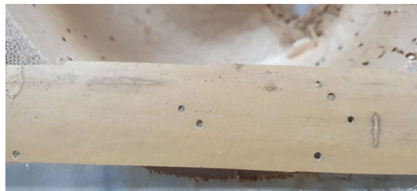
Visible exit holes (ranging from 1 to 2 mm diameter) caused by powder beetle.
